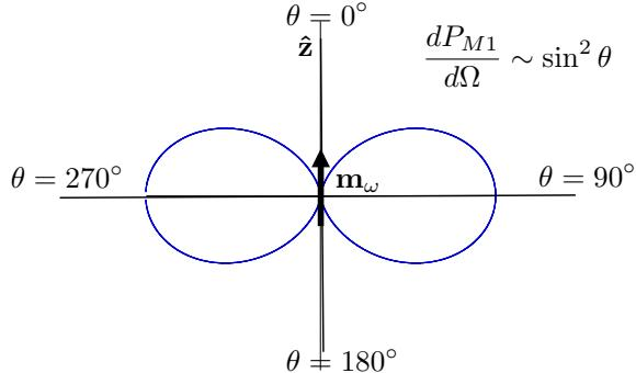
The power distribution is as shown on the left. The distribution is rotationally symmetric about the  $\hat{\mathbf{z}}$  axis. Most of the power is directed outwards into the  $xy$  plane  $\perp \mathbf{m}_\omega$ .
