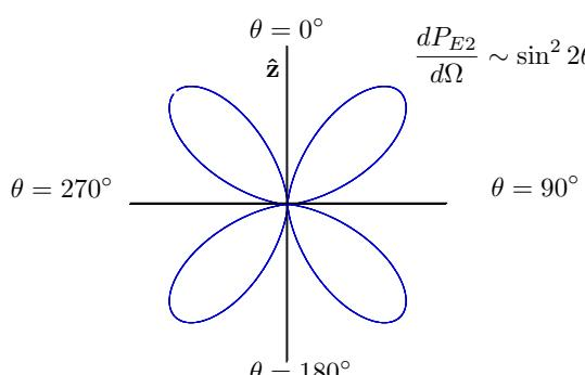
The power distribution is as shown on the left. The distribution is rotationally symmetric about the  $\hat{\mathbf{z}}$  axis. Most of the power is directed at  $\pm 45^\circ$  to the  $\hat{\mathbf{z}}$  axis.
