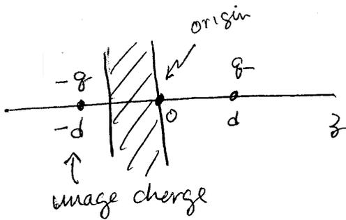
We want  $\vec{E}$  to be normal to surface on right hand side where  $q$  is. The way to do this is to put  $-q$  a distance  $-d$  behind this surface, exactly as we did for the infinitely thin plane in lecture - the finite width  $w$  here does not effect anything!
