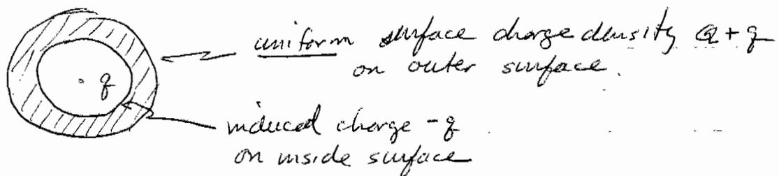
Distributing the charge in this way creates no additional  $\vec{E}$  fields in the interior - it has no effect on the force on  $q$  or on the induced  $\sigma$  on the inner surface. All it does is add a constant to the potential.
