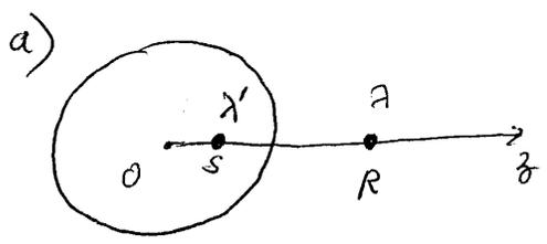
try to place image line charge λ' at distance s from origin as shown.
