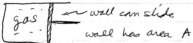
If the chamber is thermally insulating so no heat is added or taken out, and the gas is allowed to expand by moving the piston wall a distance  $\Delta x$ , then the work done by the gas on the wall is  $F^{\text{total}} \Delta x = p A \Delta x = p \Delta V$  where  $\Delta V = A \Delta x$  is the change in volume.
