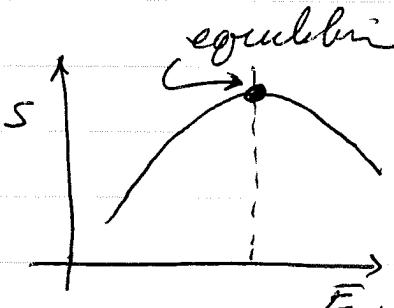
System is in equilibrium when the two subsystems have the same temperature.
