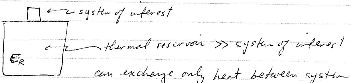
$$\left(\frac{\partial E_R}{\partial S_R}\right)_{V,N} = T_R$$
