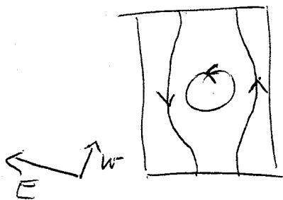
that ~~it is the~~ <sup>right</sup> hand open orbits moving along  $+\hat{k}_y$  that absorb energy, i.e.  $\vec{w} \cdot \vec{\Delta k} > 0$  for these orbits, while  $\vec{w} \cdot \vec{\Delta k} < 0$  for left hand open orbits moving along  $-\hat{k}_y$ .
