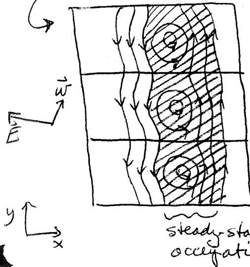
when  $\vec{E} \neq 0$ , in steady state, there will be an imbalance in occupation of open orbits, so that those orbits which ~~not~~ absorb energy from the E-field have a larger population than those which lose energy to the field. ( $\vec{E}$  field heats up metal!)
