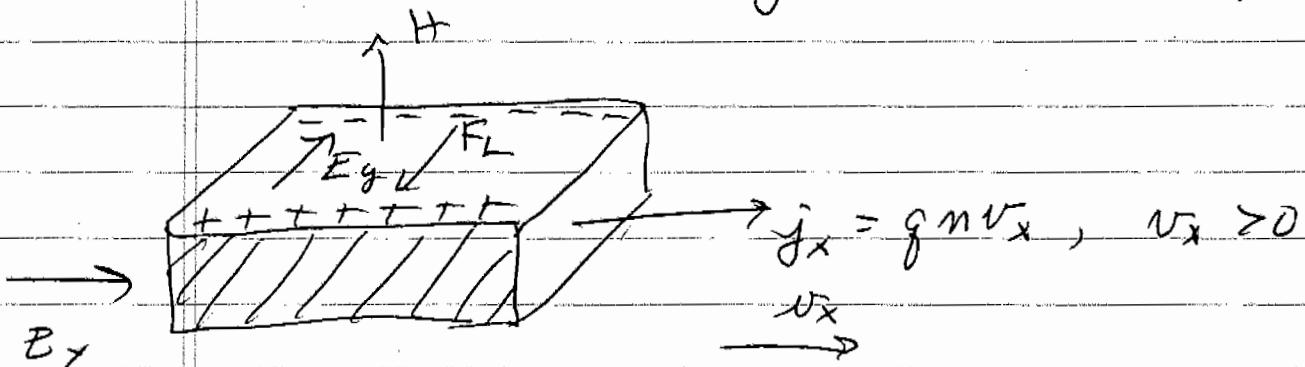
$F_L$  deflects the mobile positive charges carrying the current and positive charge builds up on the shaded surface
