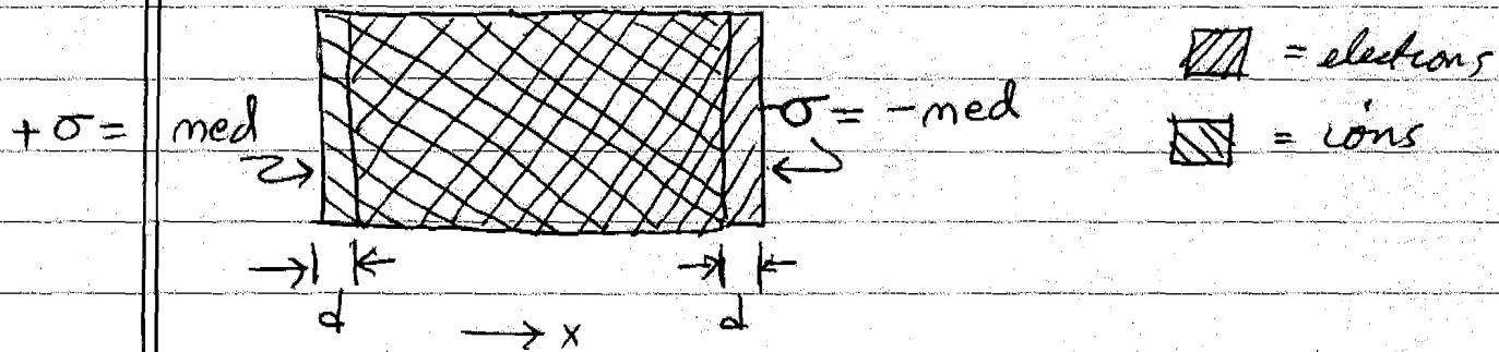
Surface charge  $\sigma$  creates electric field inside
