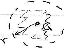
electrons get attracted to charge  $Q$  and so the average electron density about  $Q$  increases above average. The cloud of electron charge at  $Q$  "screens" the charge  $Q$ . If one computes the total charge (i.e.  $Q$  + induced electron charge) in a sphere of radius  $r$  centered on  $Q$ , this total charge decreases to zero as  $r \rightarrow \infty$ . Decay of the total charge is on length scale  $1/k_0$ .
