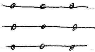
"lattice planes" - set of parallel planes containing the points of the lattice
