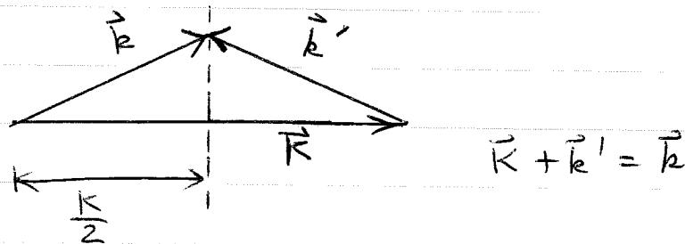
From above picture we see that there will be a Bragg peak in the diffraction pattern whenever the tip of the incident wave vector  $\vec{k}$  lies on a plane in  $k$ -space that bisects a reciprocal lattice vector  $\vec{R}$ . Such a plane in  $k$ -space is called a Bragg plane.
