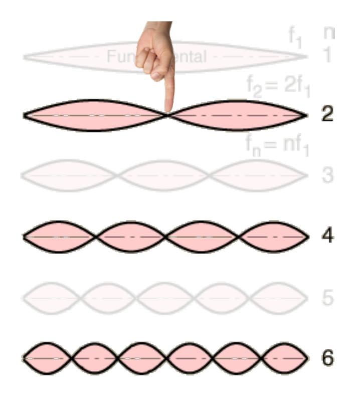
If a string is touched at its midpoint, it can only vibrate at frequencies with a node at the midpoint
