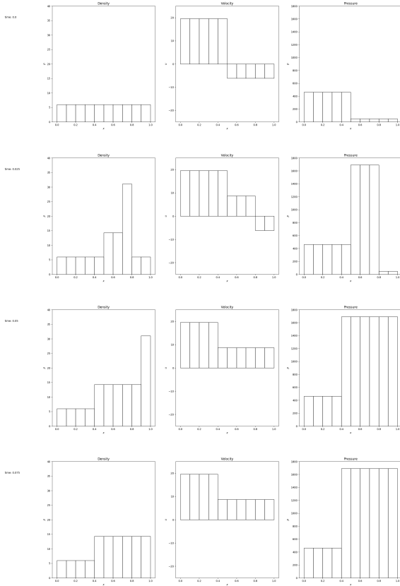
Figure 5. Test 5. Shock on both sides. Right shock is about 10 times faster than the left one.
